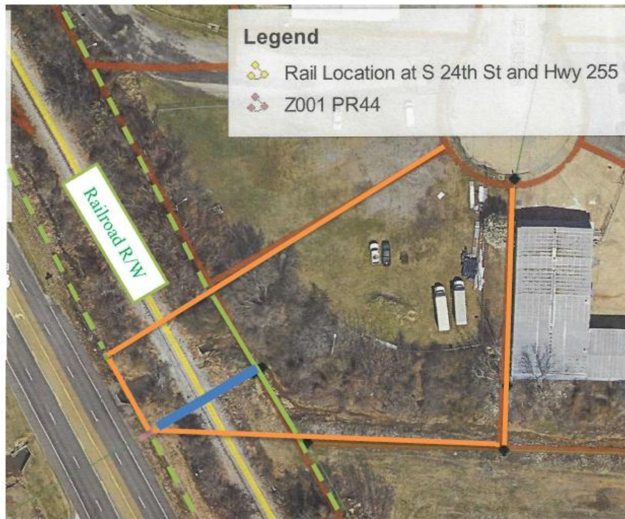
ASSEMBLED SITE AND PROPOSED EASEMENT Orange Line is Assembled Tract. Green Dash Line is Railroad R/W Blue Line is the Proposed Sewer Easement.
